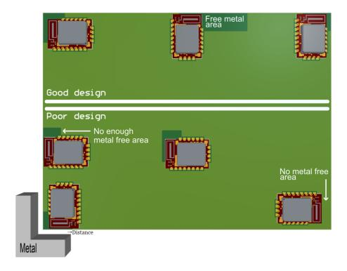
Figure 10: Placement of the module with integrated antenna
