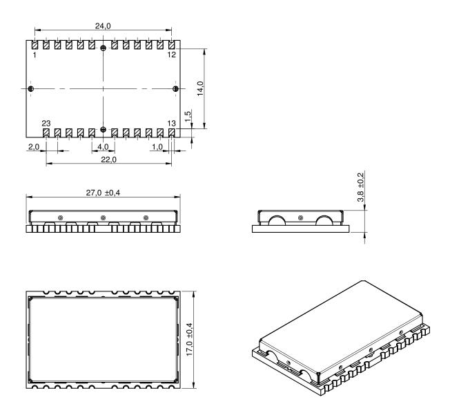
Figure 18: Module dimensions [mm]
