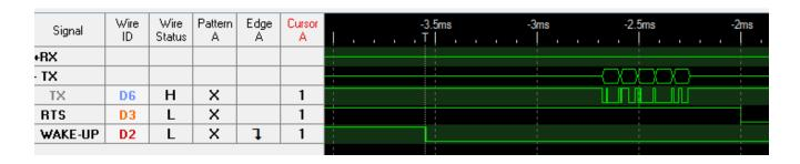
Figure 4: Wake-up from standby
