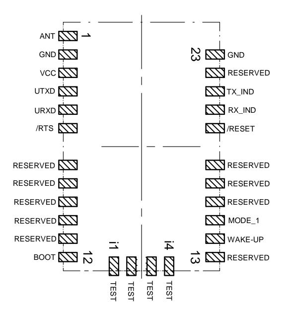
Figure 2: Pinout (top view)
