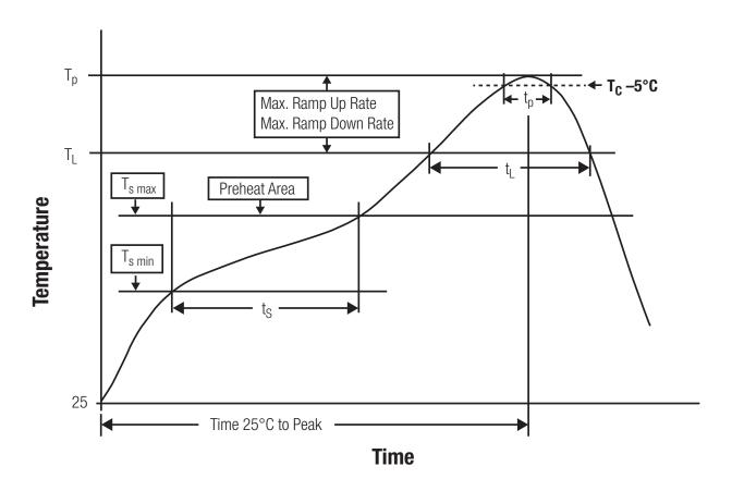
Figure 17: Reflow soldering profile
