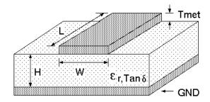
Figure 11: Dimensioning the antenna connection as micro strip
