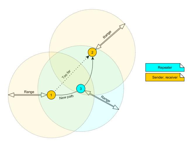
Figure 6: Range extension using several repeaters
