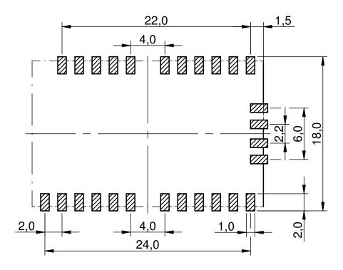
Figure 19: Footprint and dimensions [mm]
